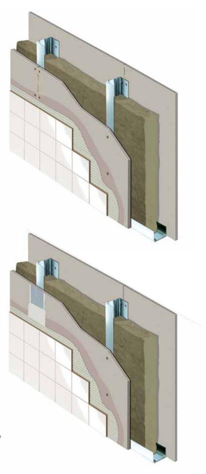
Joint treatment with Knauf AQUAPANEL® Joint Filler & Skim Coating – white and Knauf AQUAPANEL® Tape
