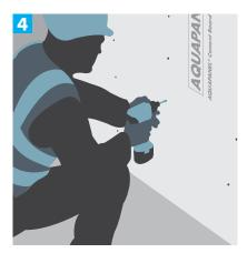
**Step 4.** Fasten the board to the framework using AQUAPANEL® Maxi Screws SN 25mm for metal studs or AQUAPANEL® Maxi Screws SN 39mm for timber. Apply the boards with the Aquapanel logo facing outwards.
